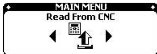
User use this function to take PUNCH out program or parameter from CNC machine and save to device
