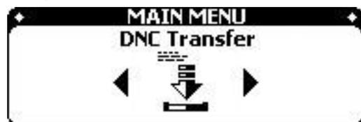
User use this function to transmit file to CNC machine in mode READ or DNC (mode Tape on Fanuc CNC)
