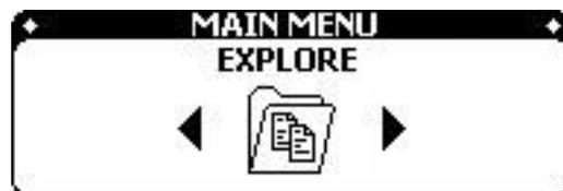
User use this function to manage files using built in memory or attached USB 2.0 device. Format, check properties, access built in memory or attached memory. For files and folders the user is able to: Read, Copy, Cut, Paste, Delete, check information of file, make new folder.
